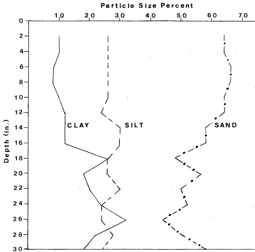
Figure 3. Mechanical Analysis for Location Three
