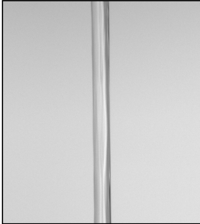
Figure 4.1 A round nonturbulent liquid jet in still air (test conditions: Water, d_j = 1 mm, We_G = 0 , Re_L = 30,000 , and q = \infty ).
