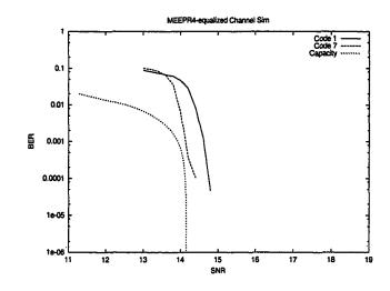
Figure 8.5: BER simulation results for block size 4352 codes over MEEPR4-equalized Lorentzian channel.
