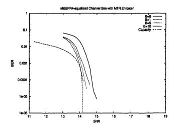
Figure 10.3: Performance of system with varying levels of MTR enforcement, without extrinsic subtraction.
