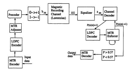
Figure 10.1: Diagram of system for PRML magnetic recording with precoder, MTR code, LDPC code and MTR enforcer.
