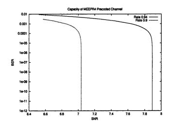
Figure 7.2: Channel capacity bound for MEEPR4 with  $1/(1 \oplus D)$  precoder.
