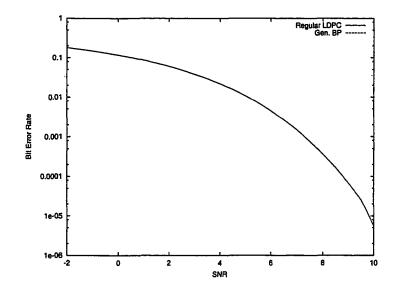
Figure 9.3: Bit error rate of ordinary BP versus generalized BP decoding of rate 2/3 code.
