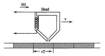
Figure 1.1: Drawing of magnetic recording head and medium.
