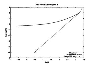
Figure 6.13:  $\log(-\log(P))$  versus  $\log(t)$  plot for max-product decoding at SNR 8 dB.
