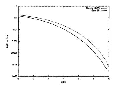
Figure 9.6: Bit error rate of ordinary BP versus generalized BP decoding of rate 1/2 code.
