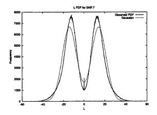
Figure 6.5: Histograms of observed L distributions versus ideal dual-Gaussian distribution for max-product decoding at 7dB SNR.
