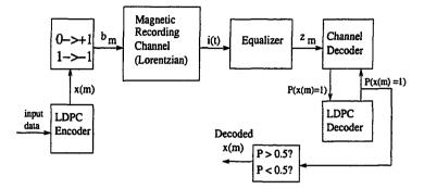
Figure 1.7: Diagram of simple system for PRML magnetic recording with LDPC error-correcting code.
