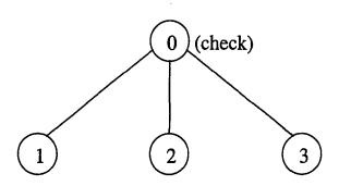
Figure 9.2: Network for our rate 2/3 parity-check code.
