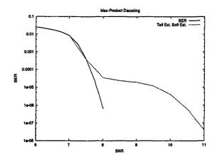
Figure 6.11: Plot of BER and tail extrapolation soft error estimate for max-product LDPC decoding.
