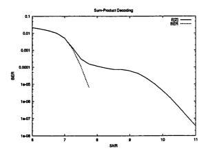
Figure 6.3: Sum-product decoding simulation results.
