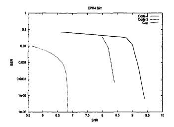
Figure 8.2: BER simulation results for block size 19340 codes over EPR4 channel.
