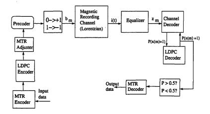
Figure 1.10: Diagram of system for PRML magnetic recording with precoder, MTR code, and LDPC code.
