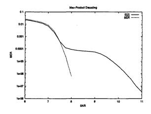
Figure 6.1: Max-product decoding simulation results.
