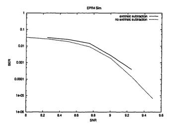
Figure 3.2: Performance of LDPC/BCJR decoder with and without extrinsic subtraction.
