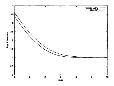
Figure 9.4: Number of iterations needed per codeword for ordinary BP versus generalized BP decoding of rate 2/3 code.
