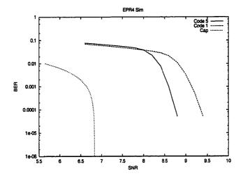
Figure 8.3: BER simulation results for block size 4835 codes over EPR4 channel.
