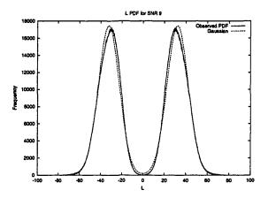
Figure 6.7: Histograms of observed L distributions versus ideal dual-Gaussian distribution for max-product decoding at 9dB SNR.
