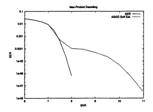
Figure 6.10: Plot of BER and asymmetric generalized Gaussian distribution soft error estimate for max-product LDPC decoding.
