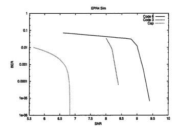
Figure 8.4: BER simulation results for block size 19340 codes over EPR4 channel.
