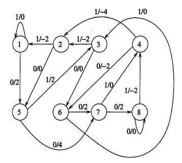
Figure 1.5: State transition diagram for EPR4 channel, mapping binary inputs to real outputs.
