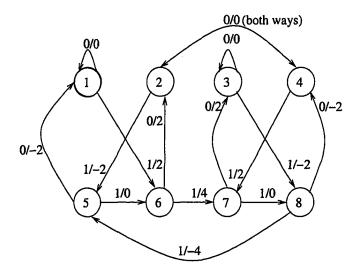
Figure 1.8: State transition diagram for precoded EPR4 channel, mapping binary inputs to real outputs.
