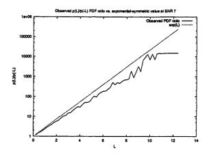
Figure 6.8: Plot of p(L)/p(-L) showing (lack of) exponential symmetry in the pdf of L.
