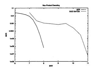
Figure 6.9: Plot of BER and generalized Gaussian distribution soft error estimate for max-product LDPC decoding.
