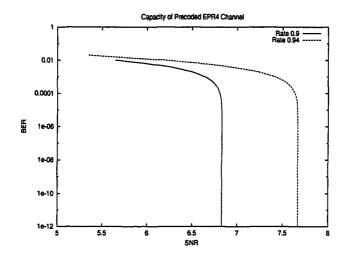
Figure 7.1: Channel capacity bound for EPR4 with  $1/(1 \oplus D^2)$  precoder.
