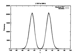
Figure 6.6: Histograms of observed L distributions versus ideal dual-Gaussian distribution for max-product decoding at 8dB SNR.
