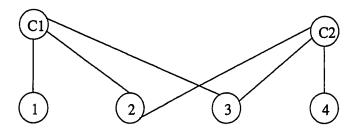
Figure 3.1: Network for a very simple LDPC code.
