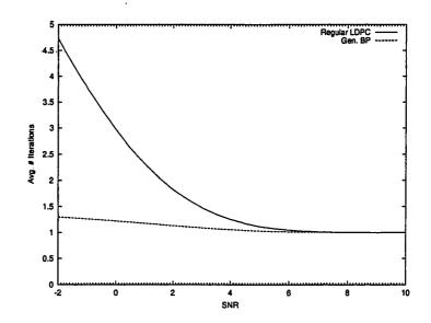
Figure 9.7: Number of iterations needed per codeword for ordinary BP versus generalized BP decoding of rate 1/2 code.
