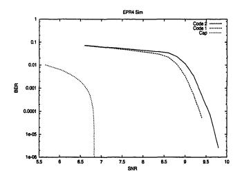
Figure 8.1: BER simulation results for block size 4835 codes over EPR4 channel.
