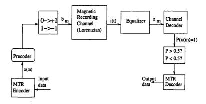
Figure 1.9: Diagram of simple system for PRML magnetic recording with precoder and MTR code.
