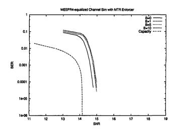
Figure 10.2: Performance of system with varying levels of MTR enforcement, using extrinsic subtraction.
