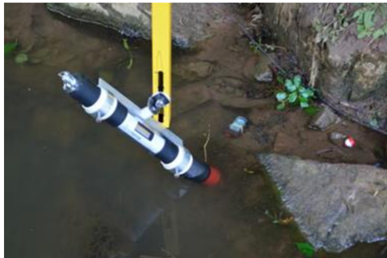
Figure 6. Example of the Benthotorch® measuring chlorophyll a in situ with water too deep to collect an algae sample using standard methods.
