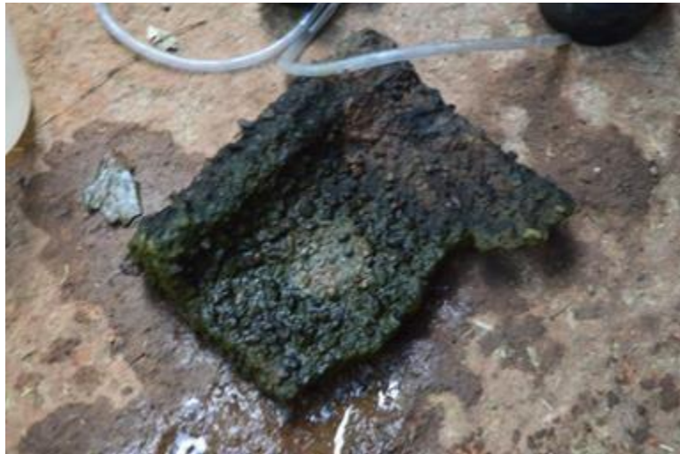
Figure 4. Example substrate too coarse for consistent Benthotorch® measurements and did not allow a good seal for a traditional algae sampler.
