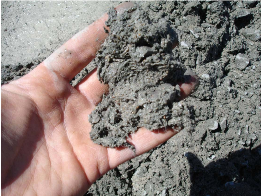
Figure 6. 16 – Sample from an Original Dry Fiber Mix at the Bridge Site
