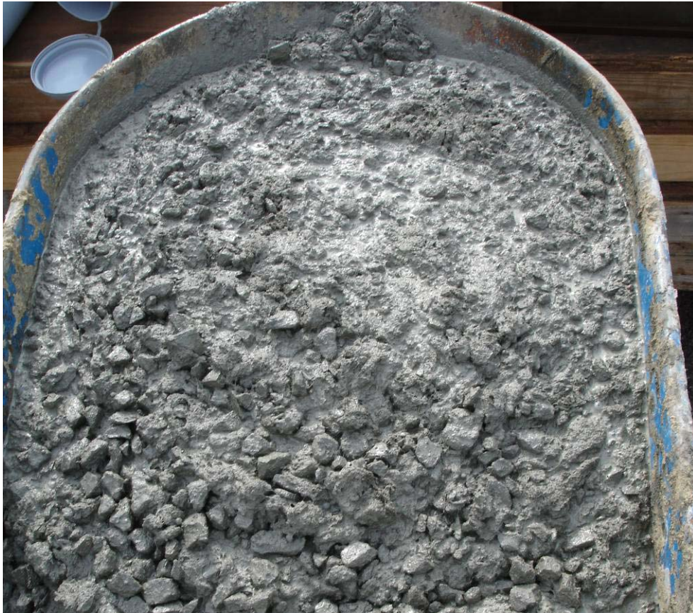
Figure 6. 17 – Sample of the Improved Fiber Mixture Used in the Construction of Span 3
