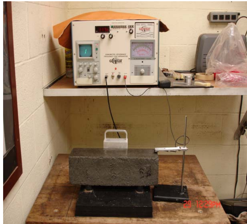
Figure 3. 8 – Transvers Frequency Reader Set Up
