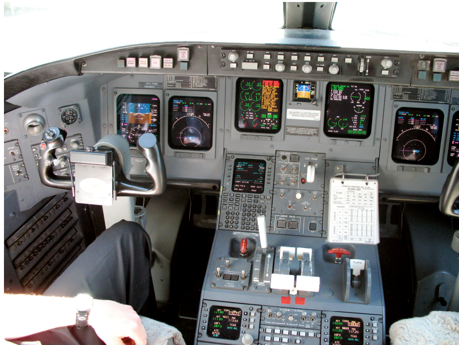
Figure 2. CRJ-200 Glass Cockpit in a Technically Advanced Aircraft Commonly (TAA) Used for Regional Airline Training.
