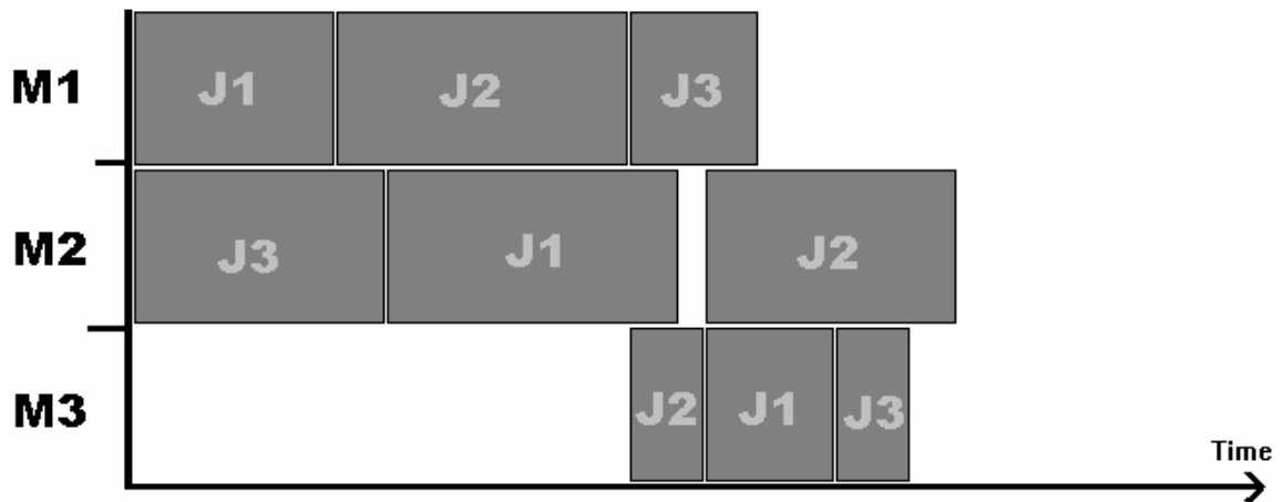
Figure 2.5: Active Schedule after Left Shifting
