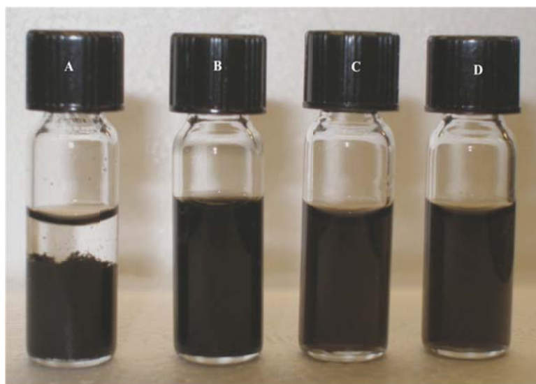
Figure 4-5: Stability of MWNT before and after surface modification (A. MWNTs; B. MWNT@PEI; C. MWNT@PEI/ssDNA; D. MWNTs@PEI/ssDNA/PVIII).
