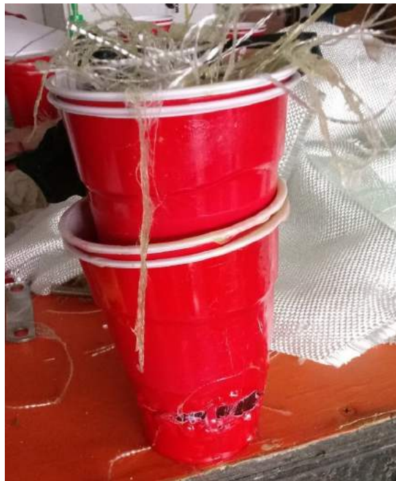
Figure 10. The effect fiberglass resin has on our mixing cups, not due to heat
