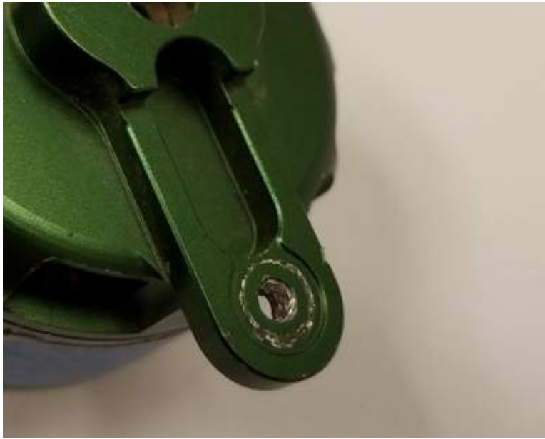
Figure 36. Stripped motor propeller hole
