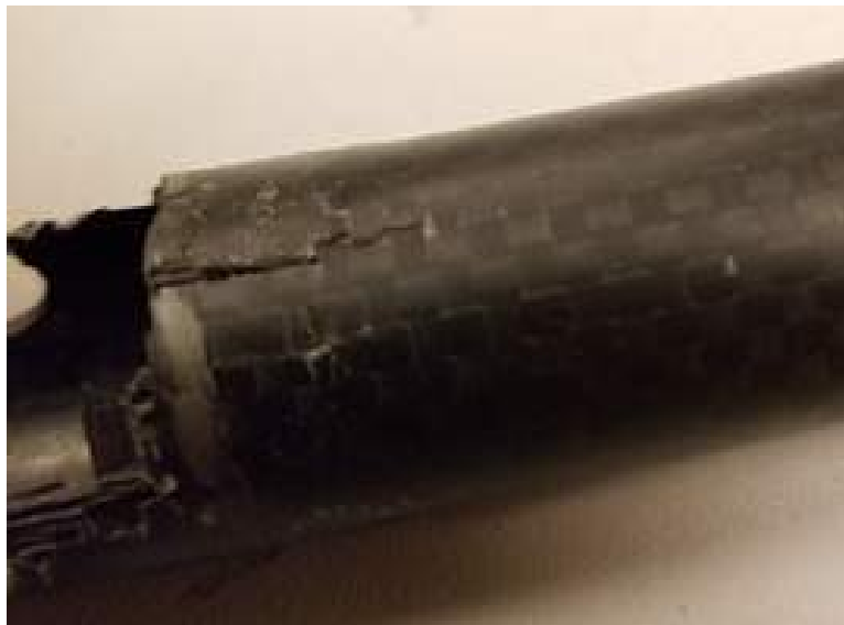
Figure 31. Cracking carbon fiber arm
