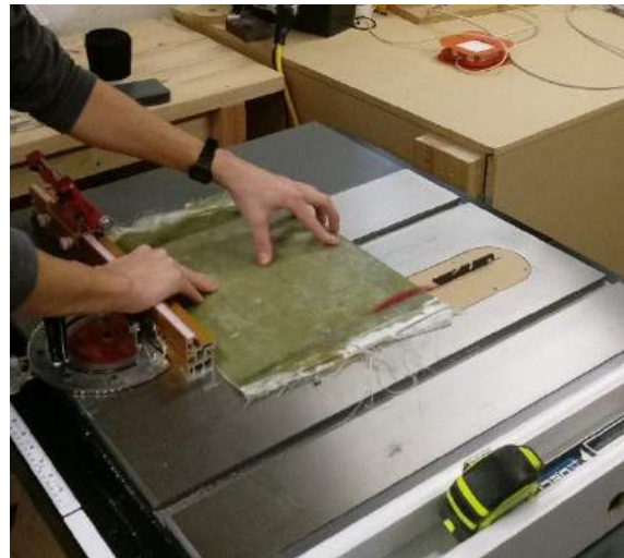
Figure 12. Edges being trimmed from the sheet
