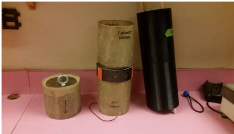
Figure 15. Piston, The Other Things altimeter bay, and 3D-printed mandrel glued together
