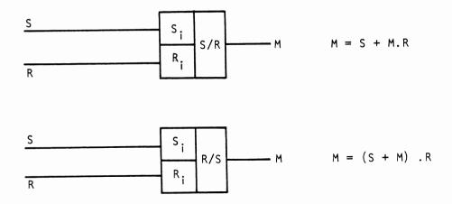
Symbol representation and logic equations are as given above, where M is the flip-flop memory.
