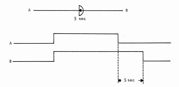
TDDE output, B is energized for n seconds even after the input signal is removed.
