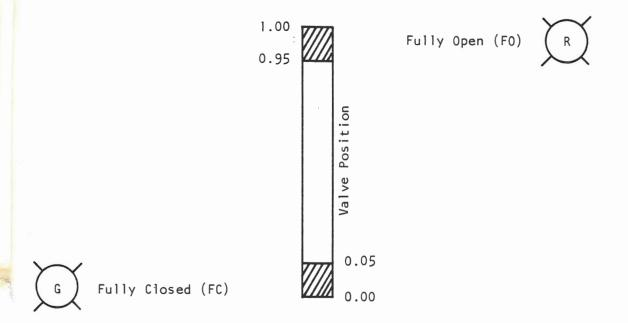
SOV status is defined as either FO (fully open) and FC (fully closed). Similarly, MOV's have defined status NFO (not fully open) and NFC (not fully closed).
