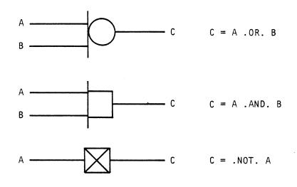
The above three symbols are used to specify logical operations OR, AND, and NOT, respectively.
