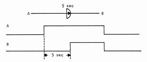
Output B is energized after a delay of n seconds after input is true and remains energized until input goes to false.
