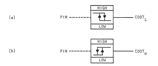
Comparator output status, COOT, is set to true when process input (a real variable indicated by the dashed line) is less than low setpoint for (a) and greater than high setpoint for (b). Logical equations determining comparator output status for (a) and (b) are:
