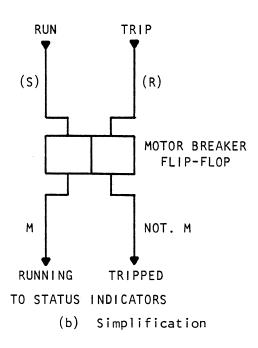
(c) Implementation: This is implemented as an R/S flip-flop with TRIP as the R-input, RUN as the S-input, and M as the Motor-Running status. Note that motor-tripped is negation of M.
