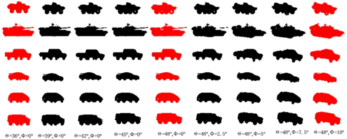
Figure 6.3: Shape interpolation on the view manifold, where the left, middle and the right ones indicates the training shapes, and others are the interpolation between those training views from left to right. The first and second training shapes are 12^\circ away from each other along the azimuth angle, and the 2nd and 3rd ones are 10^\circ along the elevation angle.
