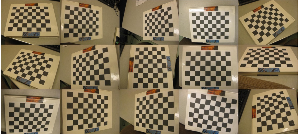
Figure 3.5: Image of pattern board for intrinsic camera calibration.
