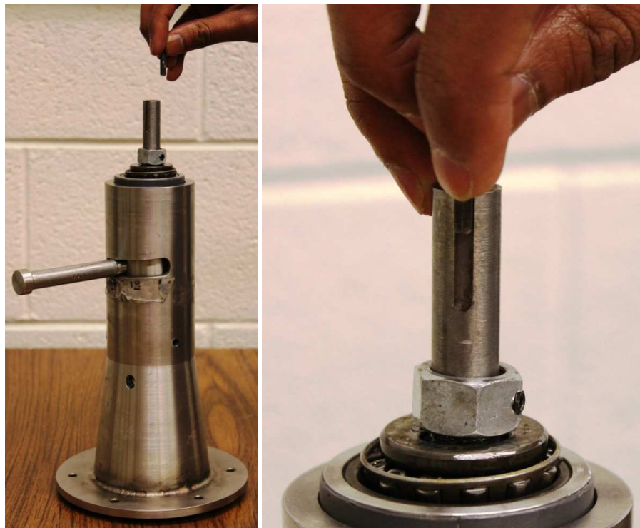
Figure 48. Installation of Rectangular Joint
