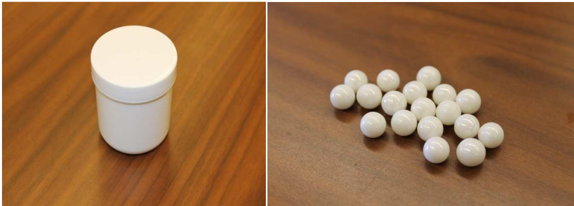
Figure 4. Plastic Cup (left) and Balls (right) for Grinding Feed
