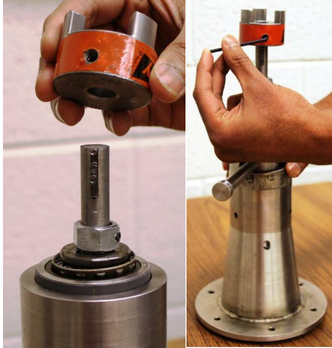
Figure 49. Installation of Lovejoy Coupling
