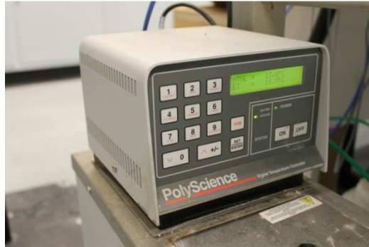
Figure 9. Poly Science Water Circulating Heating System
