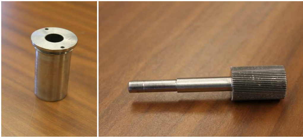
Figure 6. Serrated Cylinder (Left) and Rotating Shaft (Right)
