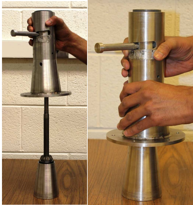
Figure 45. Installation of the Cone and Shell
