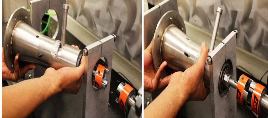
Figure 51. Installation of Reactor Assembly to the Motor
