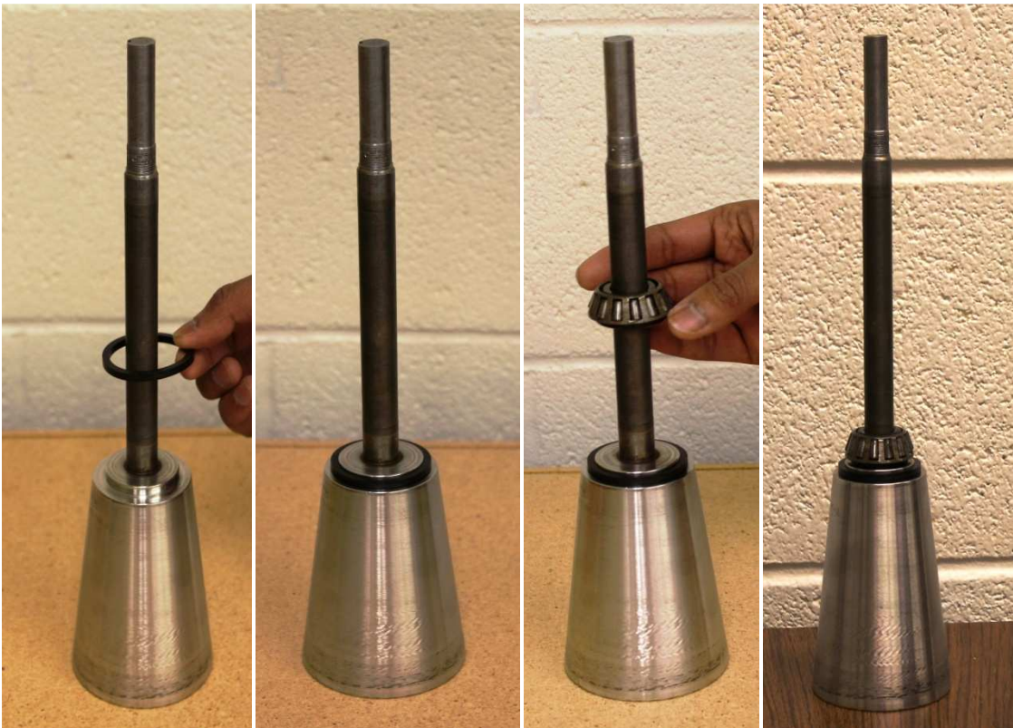
Figure 43. Installation of the Cone
