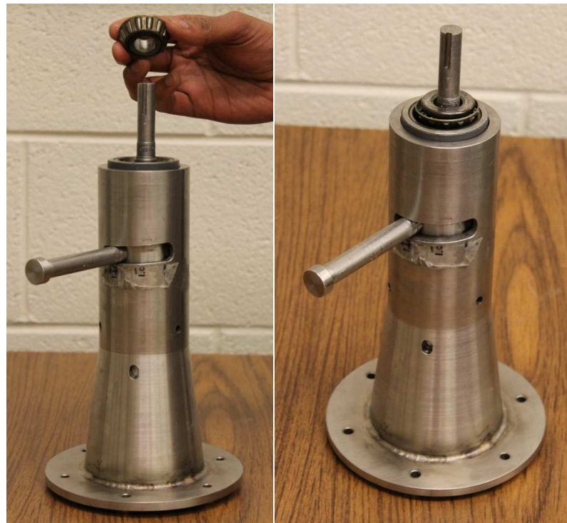
Figure 46. Installation of Tapered Bottom Bearing
