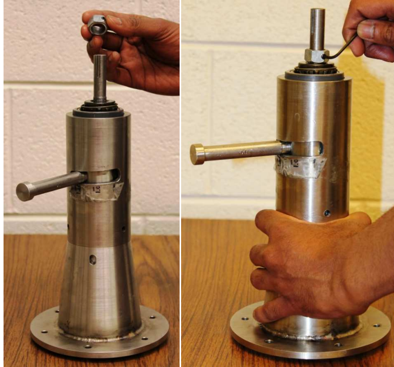
Figure 47. Installation of Nut and Set Screw
