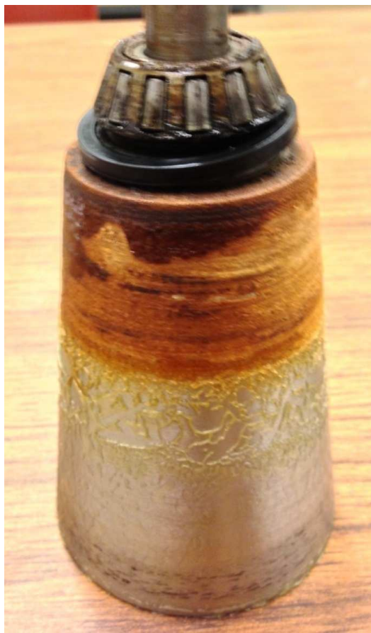
Figure 26. Burnt Mashed Potato Layer over the Cone Surface
