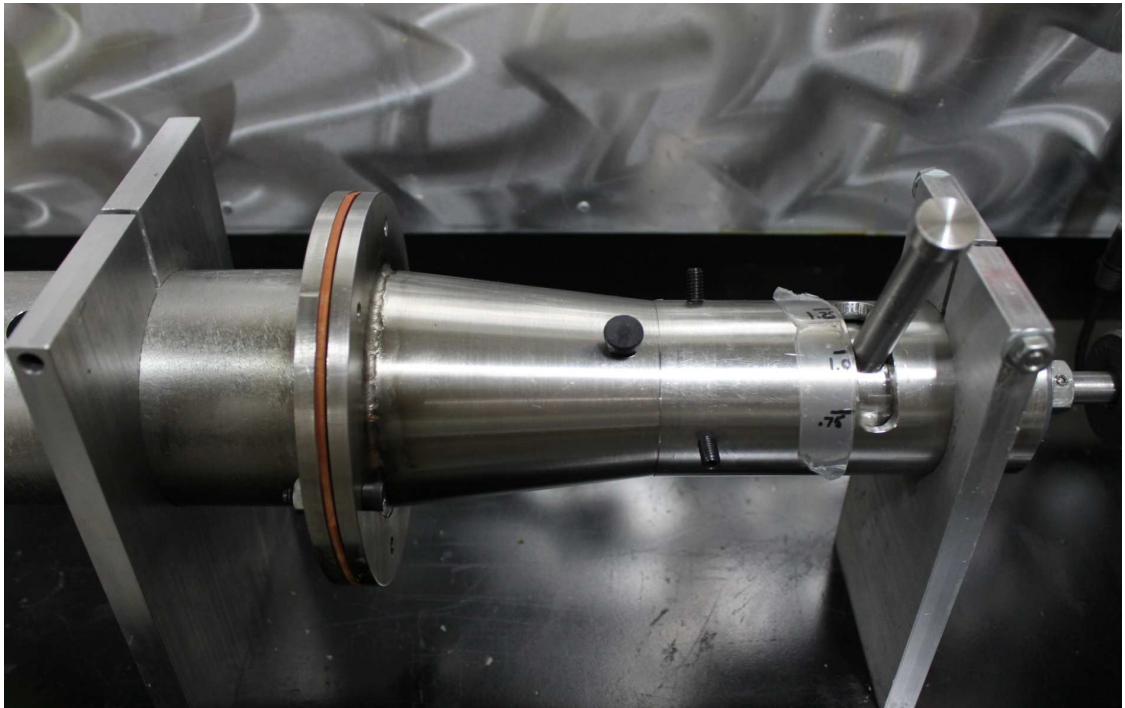
Figure 18. A Typical Setup of the Cone inside the Housing with Spacing Controller and Outlet Cork (Black)
