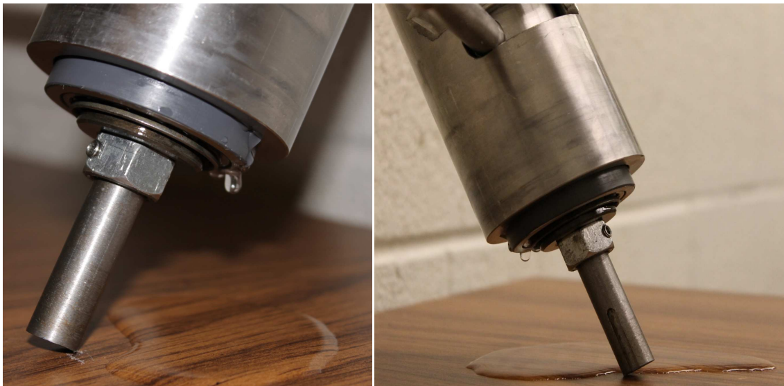
Figure 37. Water Leak from the Reactor when Charged
