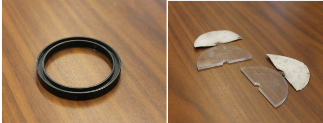
Figure 7. Black Rubber (Left) and Plastic Semi-Circular Plate with Filter Paper (Right)
