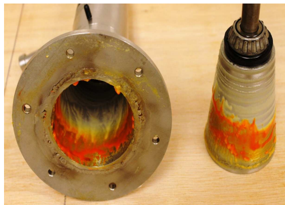
Figure 33. Vegetable Dye Passing through the Reactor to Determine Flow Pattern
