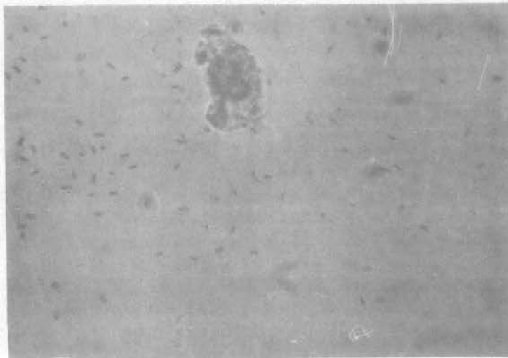
FIGURE 41 PHOTOMICROGRAPH OF A SLUDGE FROM CONTINUOUS FLOW UNIT BEFORE NaCl SHOCK. (x 2620)
