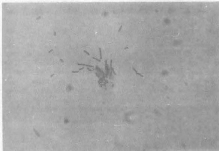
FIGURE 43 PHOTOMICROGRAPH OF SLUDGE FROM CONTINUOUS FLOW UNIT 24 HOURS AFTER BEING RETURNED TO FRESH WATER WASTE (x 2620)
