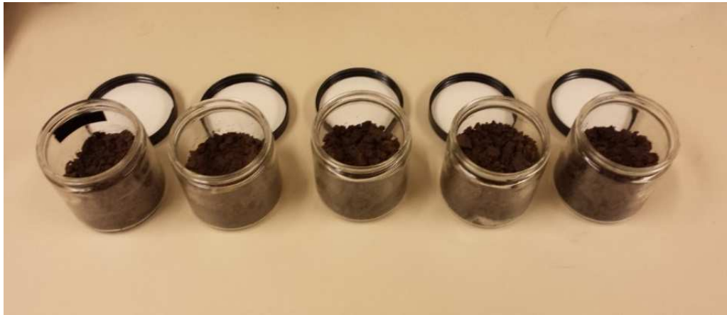
Figure 3.3. Preparation for Filter Paper Test
