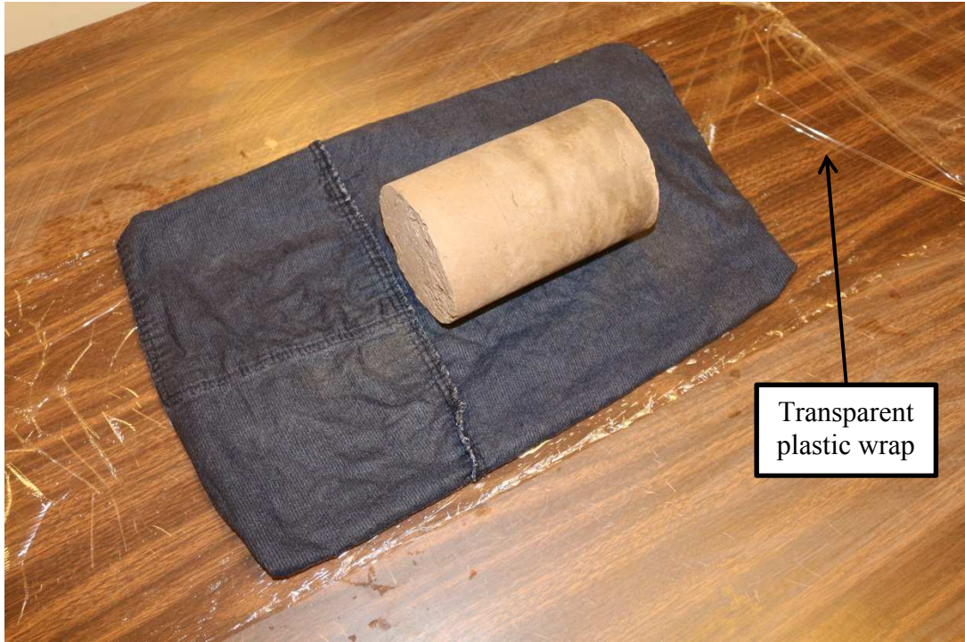
Figure 3.9. Placement of Soil Specimen
