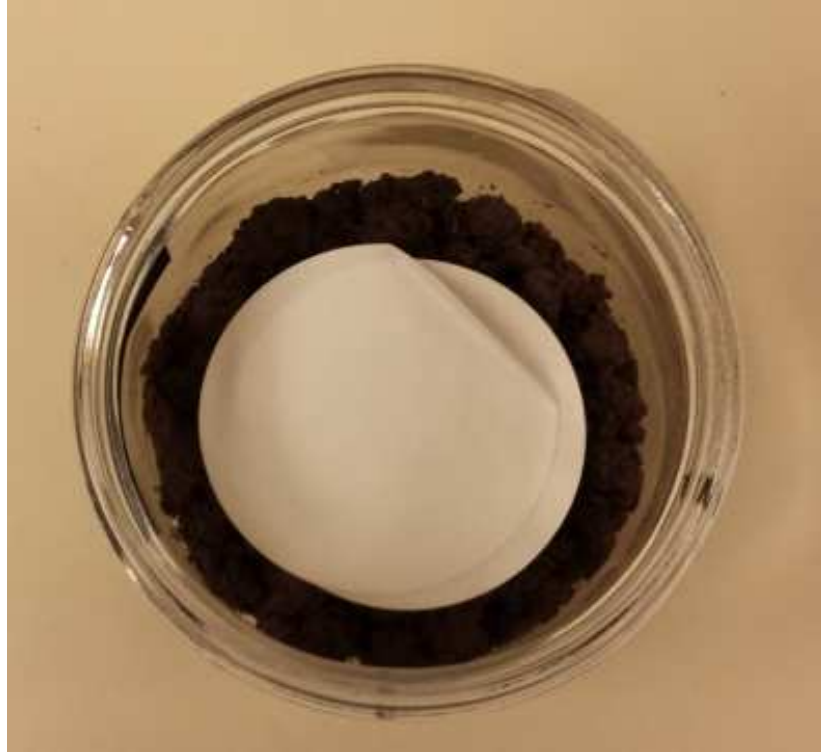
Figure 3.6. Installing Filter Papers for Suction Determination
