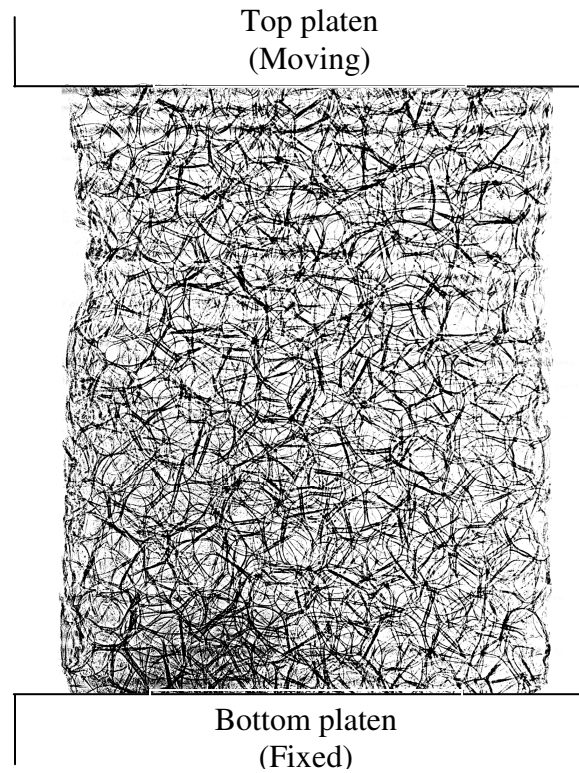
Figure 4.2 (a): Typical radiography image showing the entire foam material
