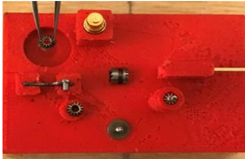
Figure 50: Gripper picking up a millimeter sized gear.
