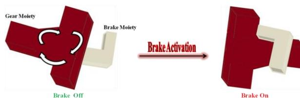
**Figure 1.4.** Conceptual depiction of the operation of a molecular brake.
