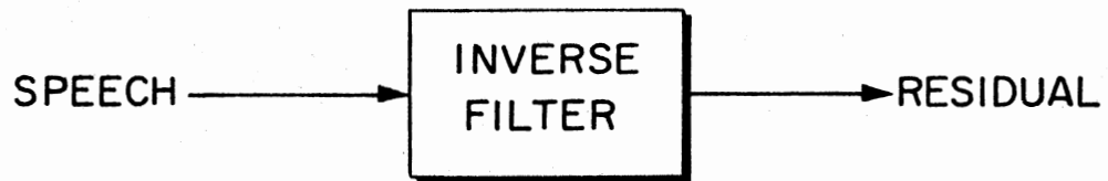
Figure 3. Prediction Residual Formed by Speech Through an Inverse Filter
