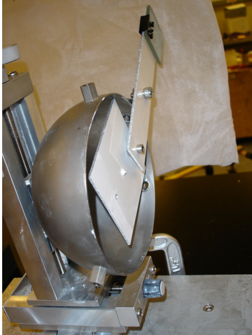
Figure 4.5: Calibration Cone for Obtaining Arrangement Parameters.
