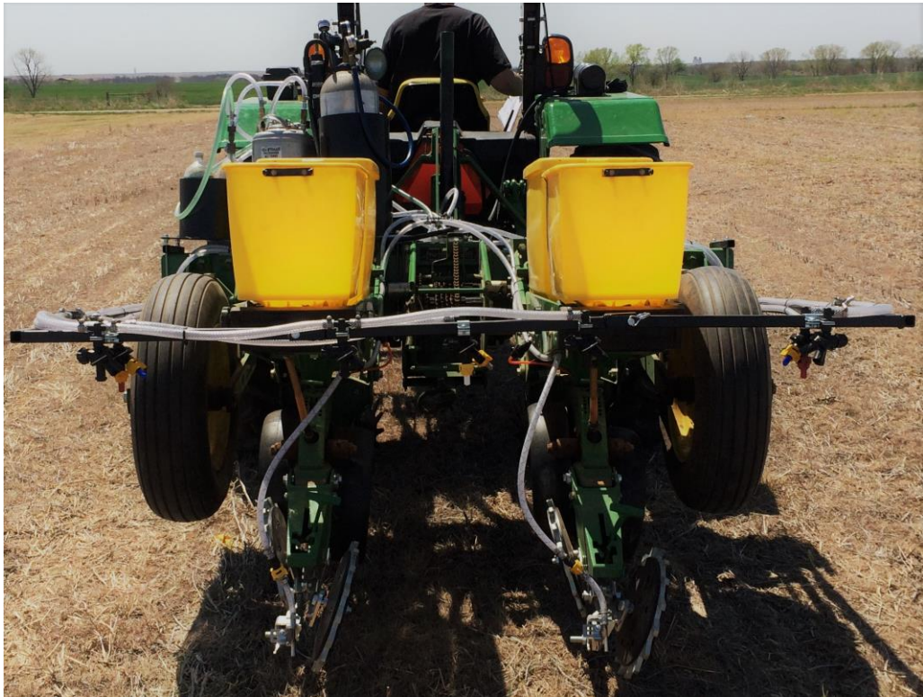
Figure 1.1 John Deere MaxEmerge two rows planter with a CO 2 system. Schaffert Seed Rebounder™ Seed Firmer was used for in-furrow liquid fertilizer applications.
