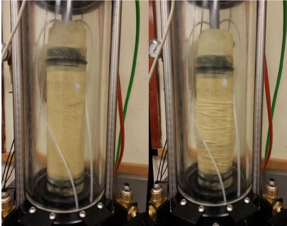
Figure 3.3. Failure of the soil sample in the testing machine
