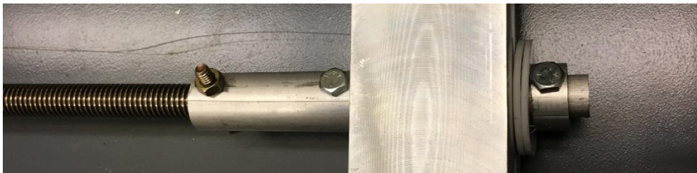
Figure 197 Finished coupling. (Front piece on the left and Back piece on the right).
