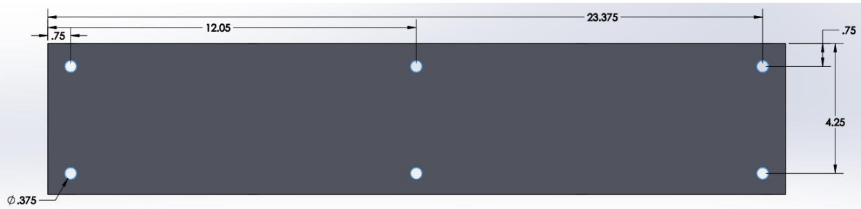
Figure 7 Dimensions of the 3/8 inch holes cut from front to back on the PVC blocks.
