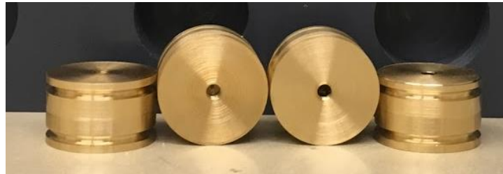
Figure 126 Finished brass stoppers.
