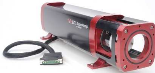
Figure 24: Programmable piston pump (ViVITRO Labs Inc., Victoria, BC, Canada) used to run the flow loop
