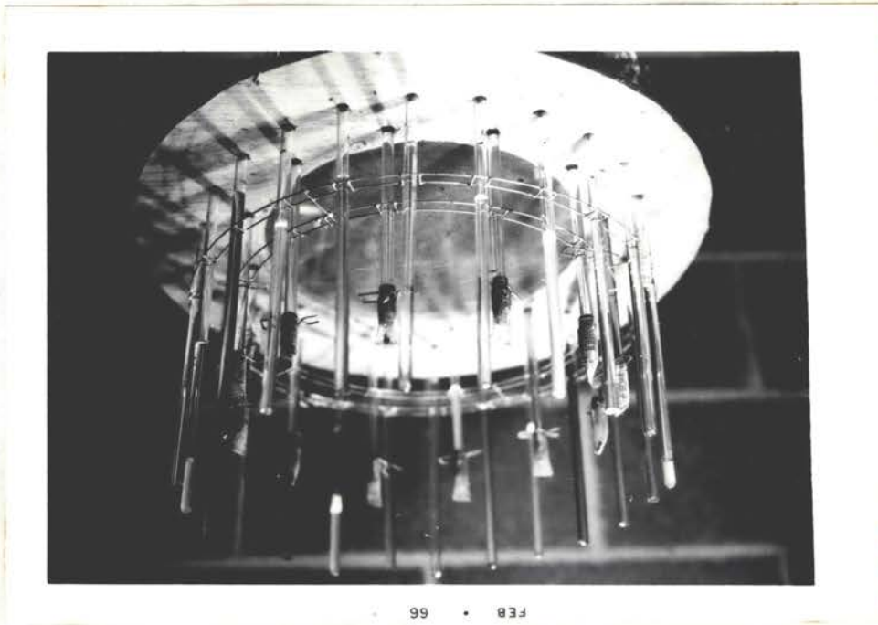
Figure 4. The bottom view of Liquid Food Experimental Unit showing consumption and evaporation check tubes
