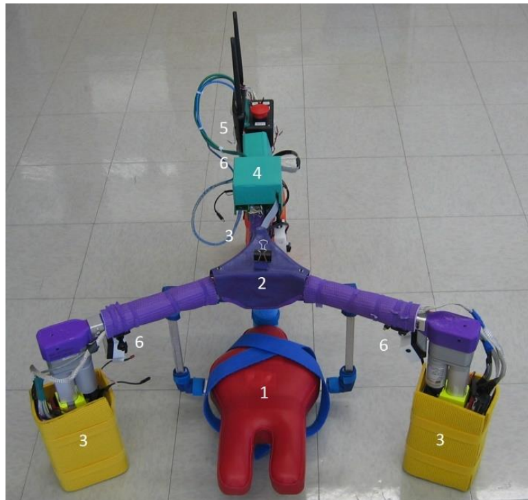
Figure 2-1. SIPPC3 front view showing locations of 1) infant support platform, 2) six-axis force-torque sensor, 3) vertical lift and Omni-wheel assemblies, 4) central processor, 5) wireless modem, and 6) GoPro video cameras.
