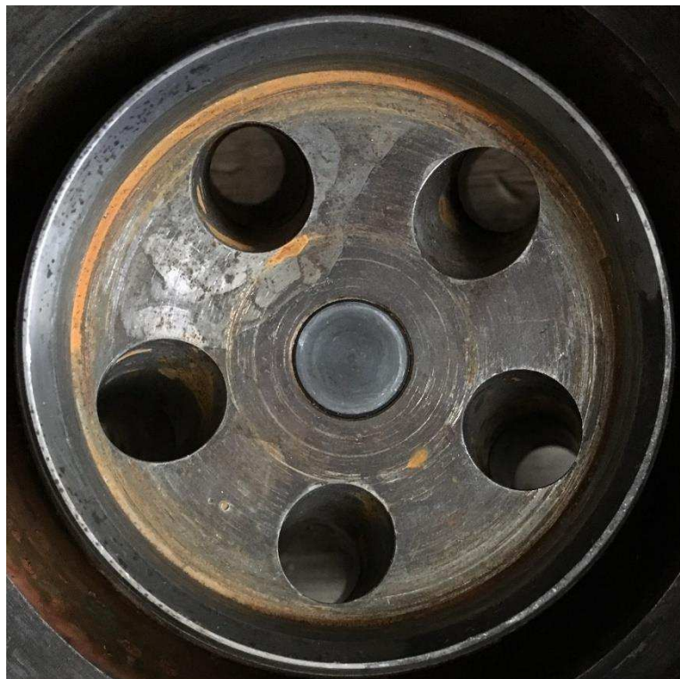
Figure 23: Slot for interrupter plate showing signs of galling
