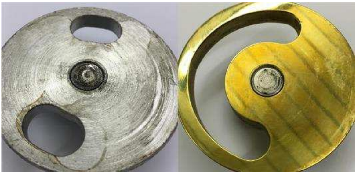
Figure 33: Interrupter plate gauging comparison. 2H plate left, 1H plate right
