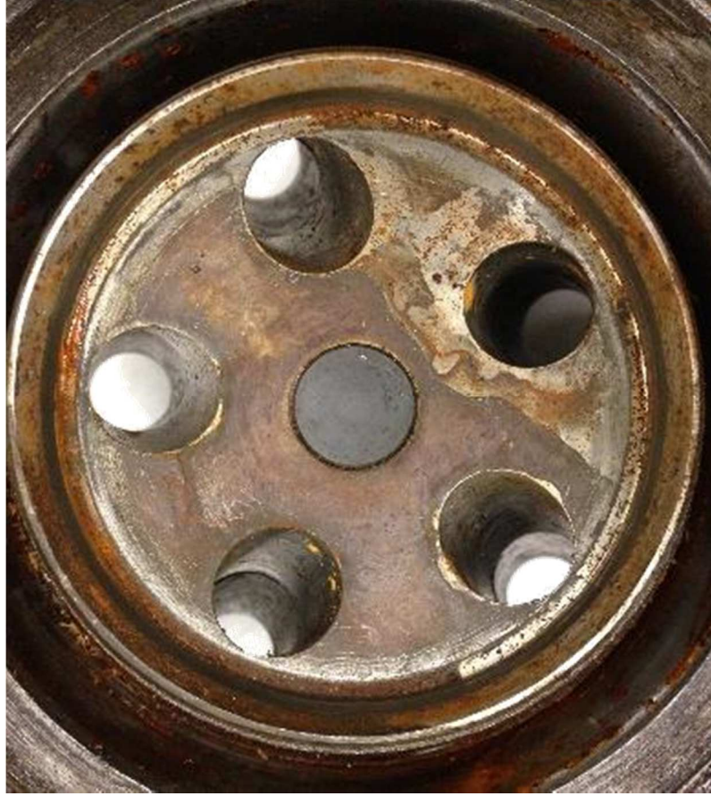
Figure 3: Internal View of Interrupter Plate Location Showing Nozzle Fluid Paths
