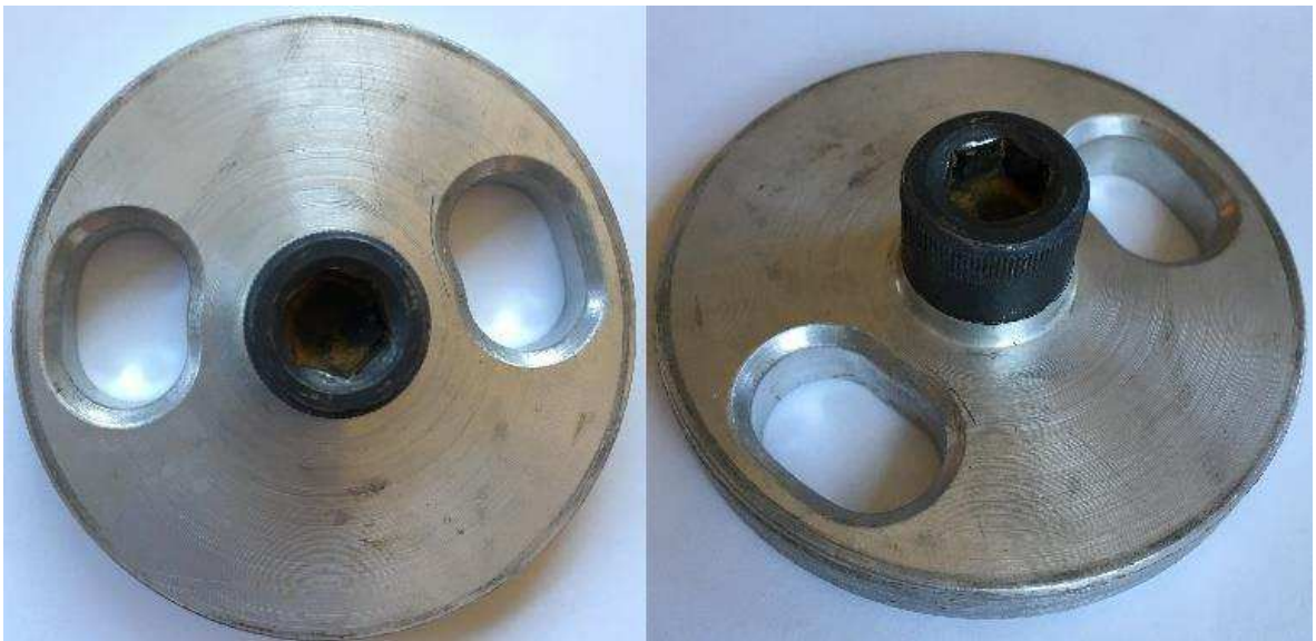
Figure 3: Internal View of Interrupter Plate Location Showing Nozzle Fluid Paths
