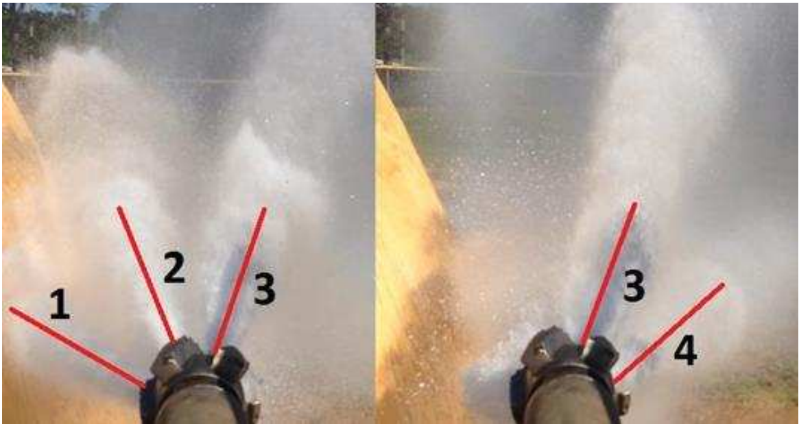
Figure 34: 1H plate changing fluid path
