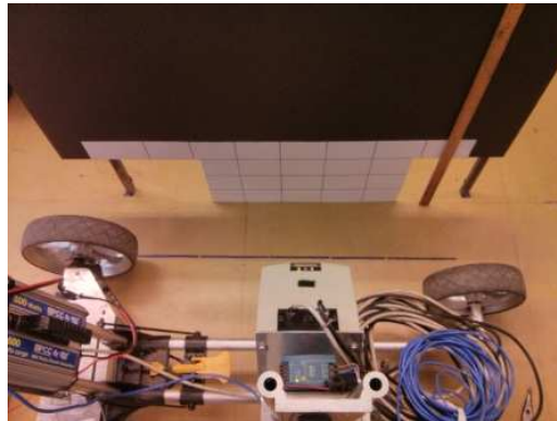
Fig. 26 In order to obtain the webcam's horizontal view angle, a paper board marked with grids was placed at three distances away from the sensors.
