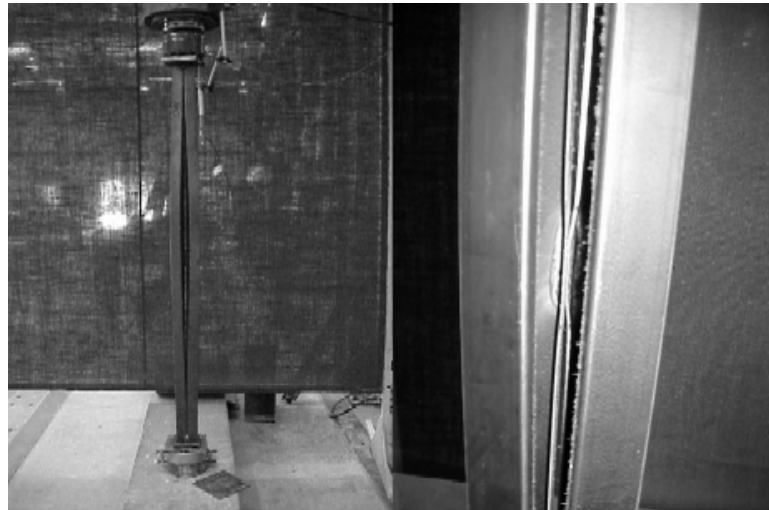
Figure 6.17 Buckling of specimen with stitch welding on one side
