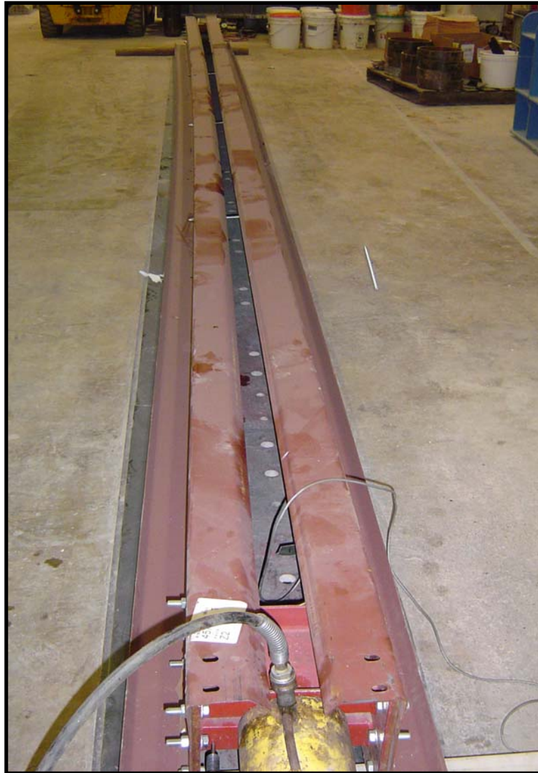
Figure 3.17 Two Purlin Test with out Lateral Restraint
