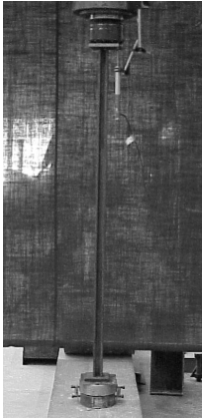
Figure 4.2 Specimen with fixed end condition ready for testing
