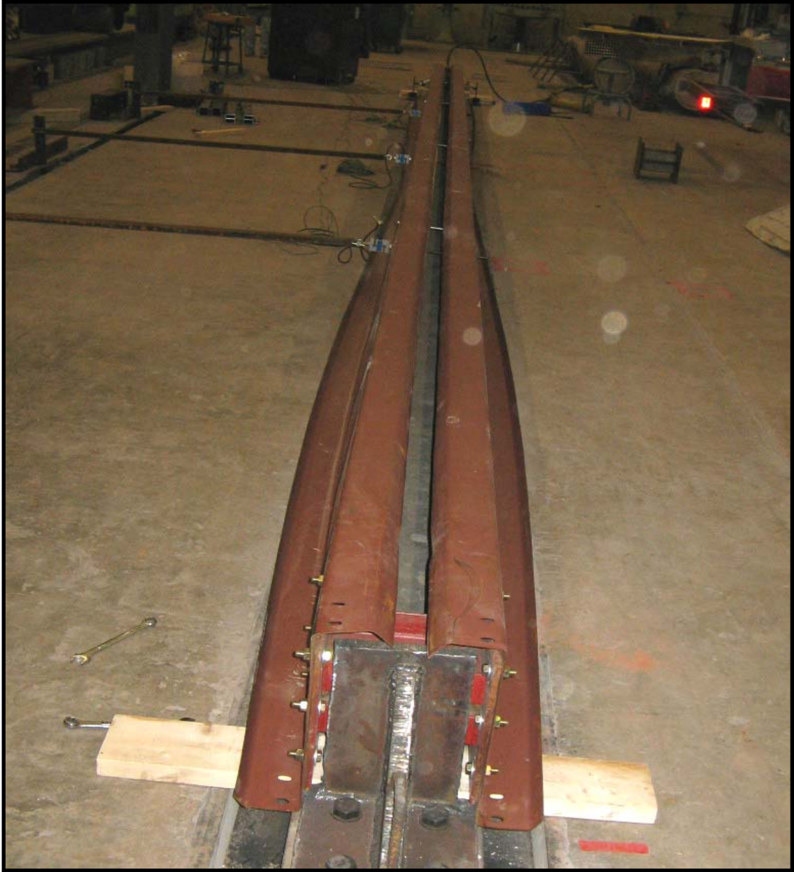
Figure 5.6 Distortional failure for restrained test of purlins with no roof panel
