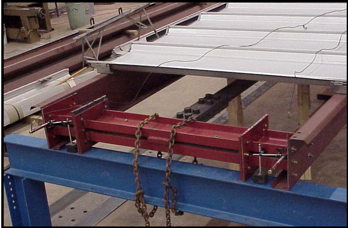
Figure 3.10 Two Purlin Test without Lateral Restraint
