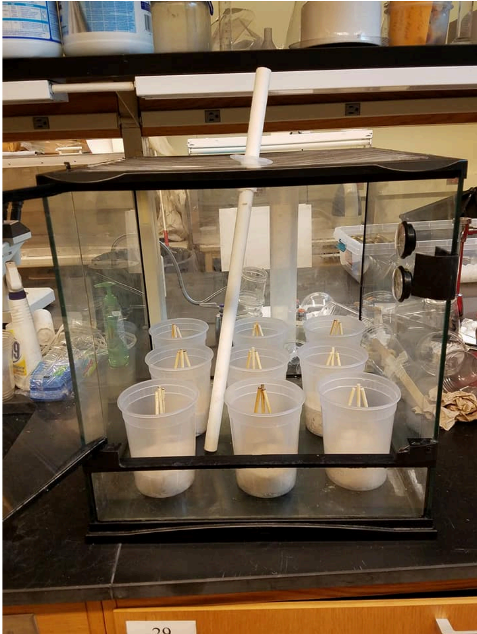
Figure 6. Photograph of flight-test terrarium. This beetles were inserted into the cups via a pvc pipe that was manipulated from outside the terrarium, in order to maintain conditions in the terrarium.
