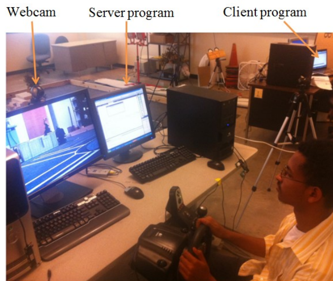
Figure 31. Manual/Autonomous switching experimental setup.
