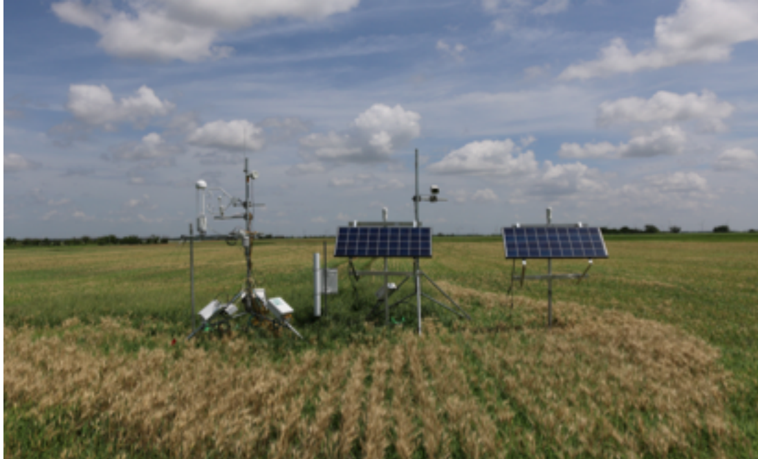
Figure 3.6: Eddy covariance flux tower setup (ICOS).
