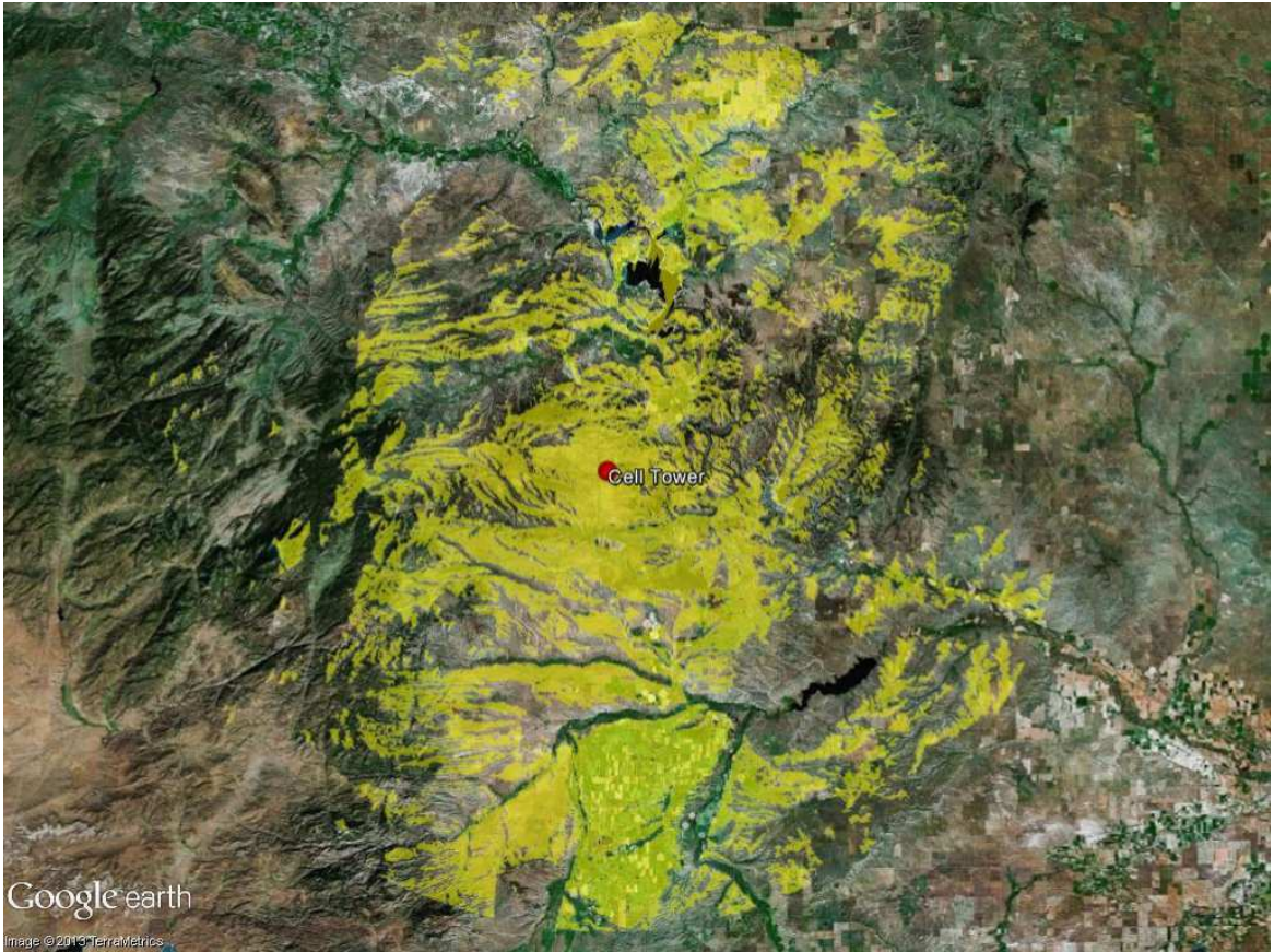
Figure 6. Displays cellular signal coverage gaps due to terrain masking in a mountainous region. Received from J. Ogden courtesy of the Civil Air Patrol. Printed with permission.
