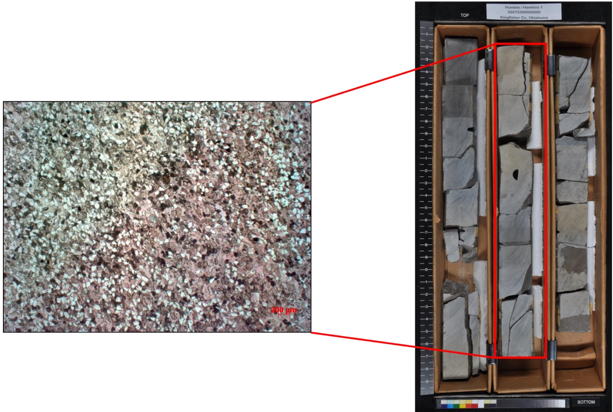
Figure 11—Calcitic siltstone in thin section (left) and whole core (right).
