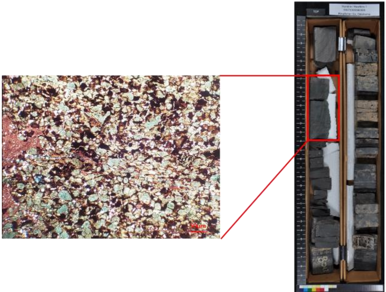
Figure 15—Glauconitic siltstone in thin section (left) and whole core (right).
