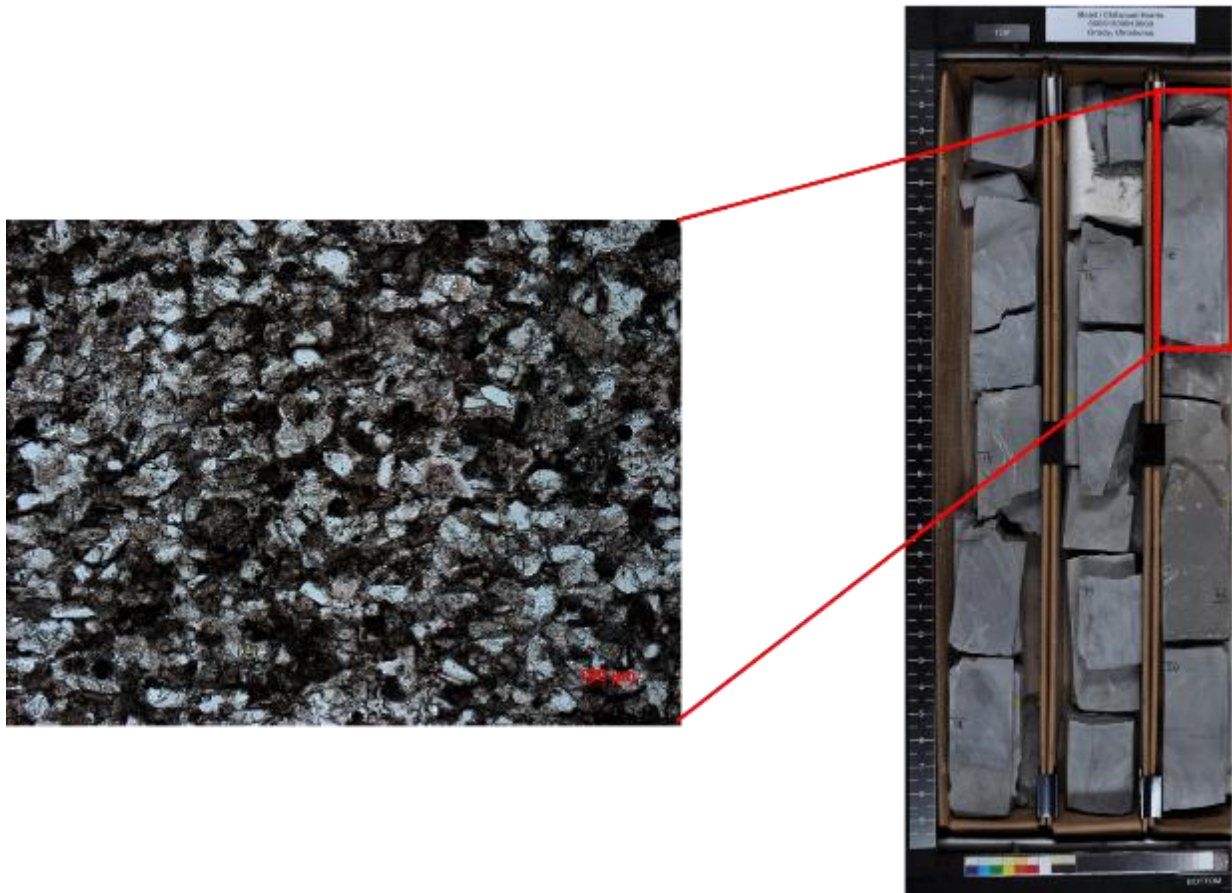
Figure 12—Argillaceous siltstone in thin section (left) and whole core (right).
