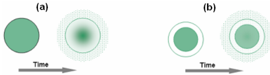
Figure 2.8. Schematic diagram of the diffusion controlled system: (a) matrix system and (b) reservoir system
