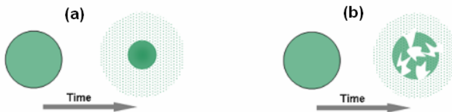
Figure 2.9. Schematic diagram of the bioerodible controlled system: (a) surface erosion system and (b) bulk erosion system.
