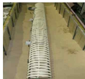
(a) Composition of sample (b) Spiral-coil type GHE setting Fig. 2 Laboratory TRT process
