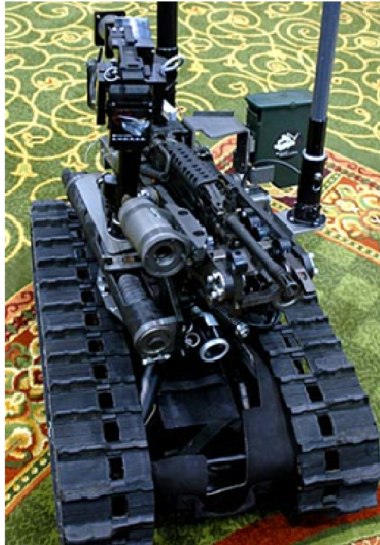
Figure 4: Foster-Miller SWORDS with M249 machine gun
