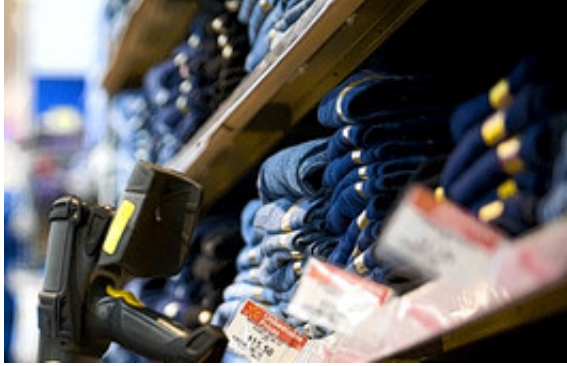
Figure 4.2: RFID handheld scanner used to read RFID tag labels for inventory checking at a Wal-Mart Supercenter. Image source: Wall street journal
