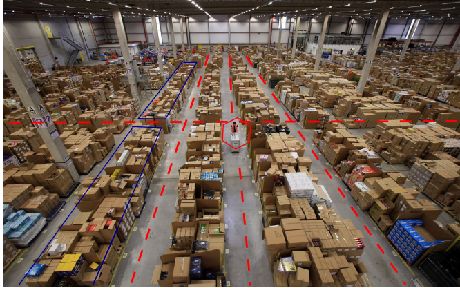
Figure 4.1: Inside an Amazon warehouse. Contiguous storage units (grids) and constrained aisle-based pathways for the reader mobility.
