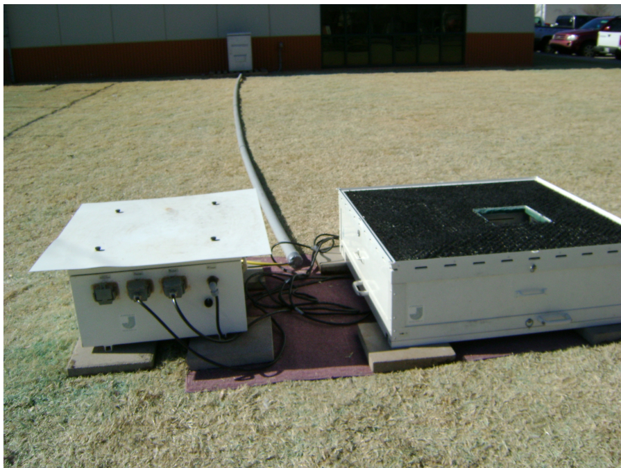
Figure 2.2: The OEU (including sensor and computer) of OU 2DVD.
