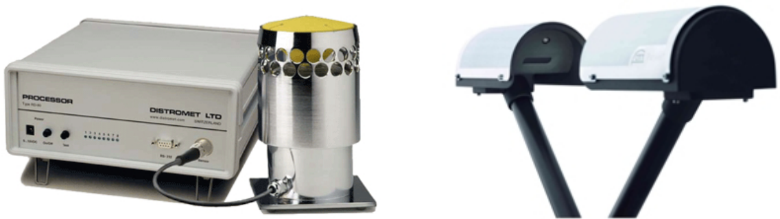
Figure 2.1: (a) Joss-Waldvogel disdrometer RD-80 (From manufacturer’s official website www.disdromet.com ). (b) Laser optical Parsivel disdrometer (From manufacturer’s official website www.ott-hydrometry.de ).
