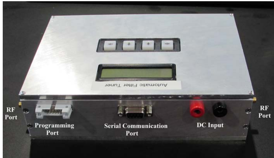
Figure 6.23: Ports of the packaged, tunable filter control system.
