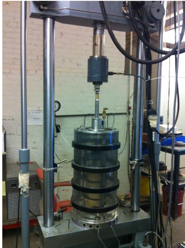
Figure 4.10 Resilient Modulus Testing in Laboratory
