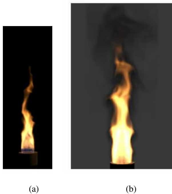
Figure 2a-b: Examples of Blue Core and Rising Soot [Nguyen et al., 2002]
