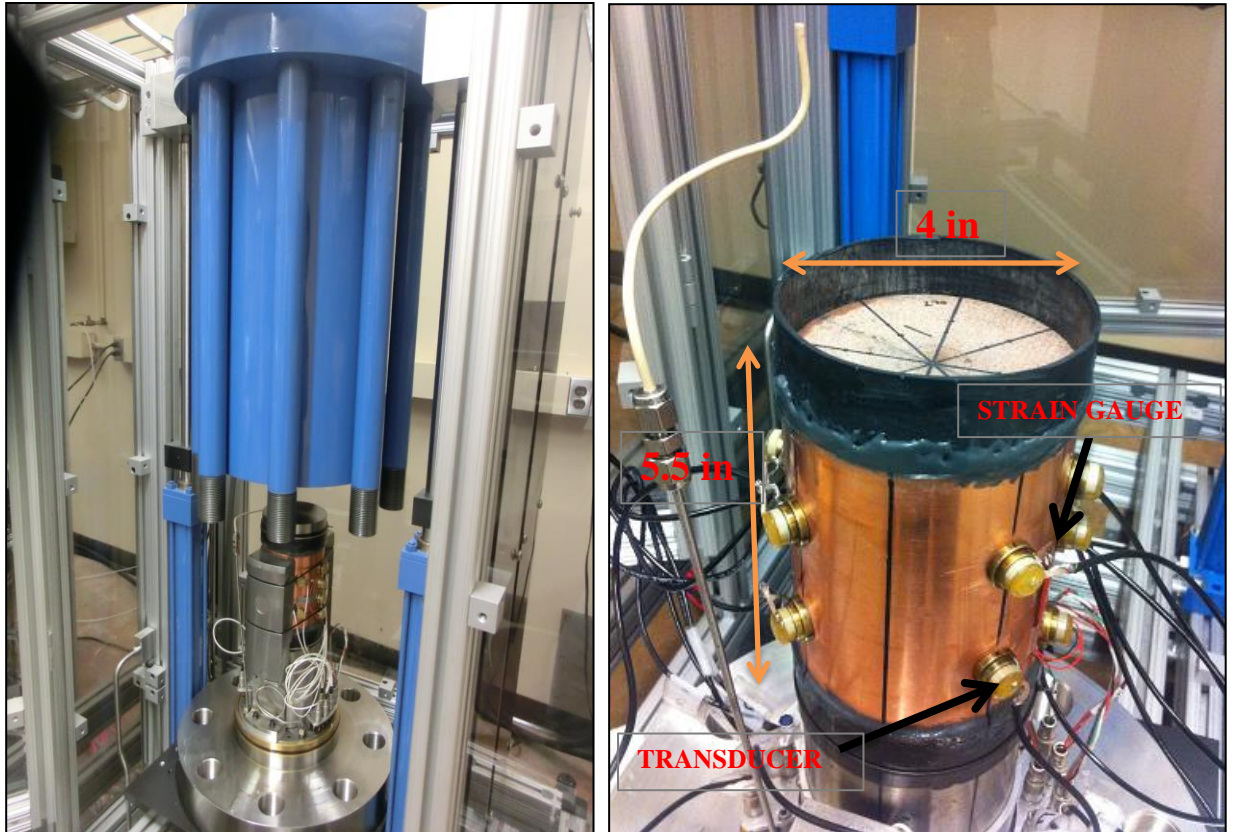
Figure 22 – Hydraulic fracturing lab experimental setup. The figure on the left shows an expanded view of the triaxial loading system with axial loading, confining vessel and flat jacks to apply transverse stress. The figure on the right shows the sample covered with copper jacket mounted on the base plate of the triaxial loading system. (Damani et al., 2012; Damani, 2013).
