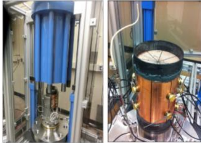
Fig. 4. Hydraulic fracturing lab experimental setup. The figure on the left shows an expanded view of the triaxial loading system with axial loading, confining vessel and flat jacks to apply transverse stress. The figure on the right shows the sample covered with copper jacket mounted on the base plate of the triaxial loading system. (Damani et al., 2012; Damani, 2013).
