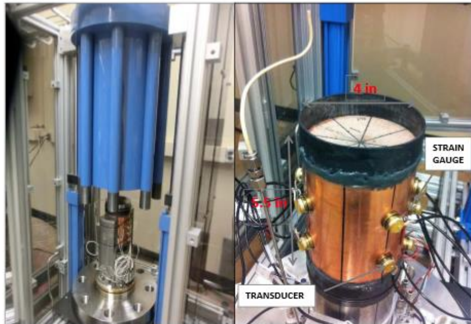
Figure 2: Hydraulic fracturing setup (courtesy of Damani et al. 2012). The figure on the left shows an expanded view of the triaxial loading system with axial loading, confining vessel and flat jacks to apply transverse stress. The figure on the right shows the sample covered with copper jacket mounted on the base plate of the triaxial loading system.
