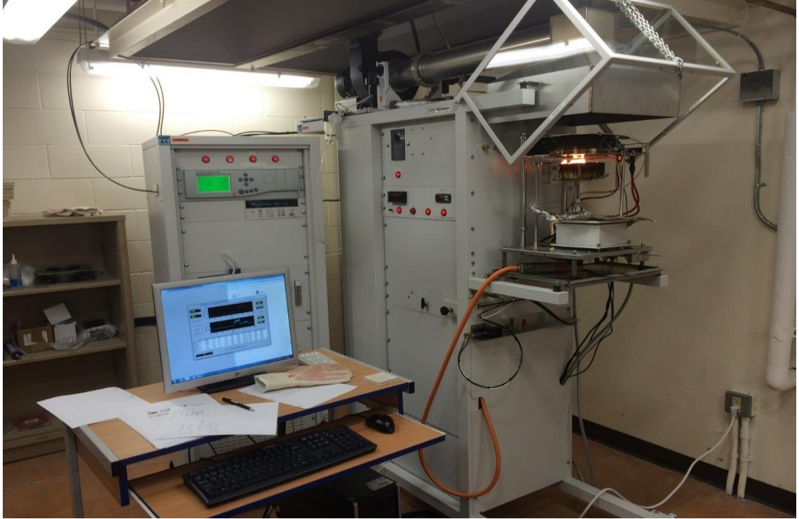
Figure 4 Cone calorimeter assembly in Fire Protection and Safety Technology Lab
