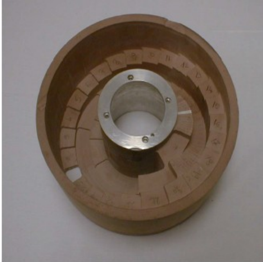
Figure 2.7: A common range modulator wheel used in proton radiotherapy. Picture taken from (Schlegel et al., 2006).
