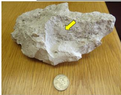
High-porosity, low density Tripolitic Chert core and rock samples
