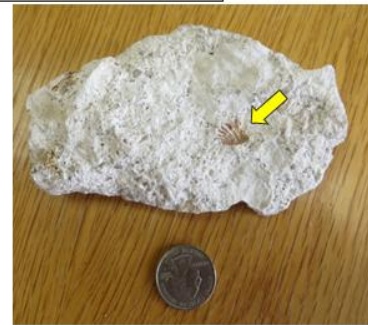
High-porosity, low density Tripolitic Chert core and rock samples
