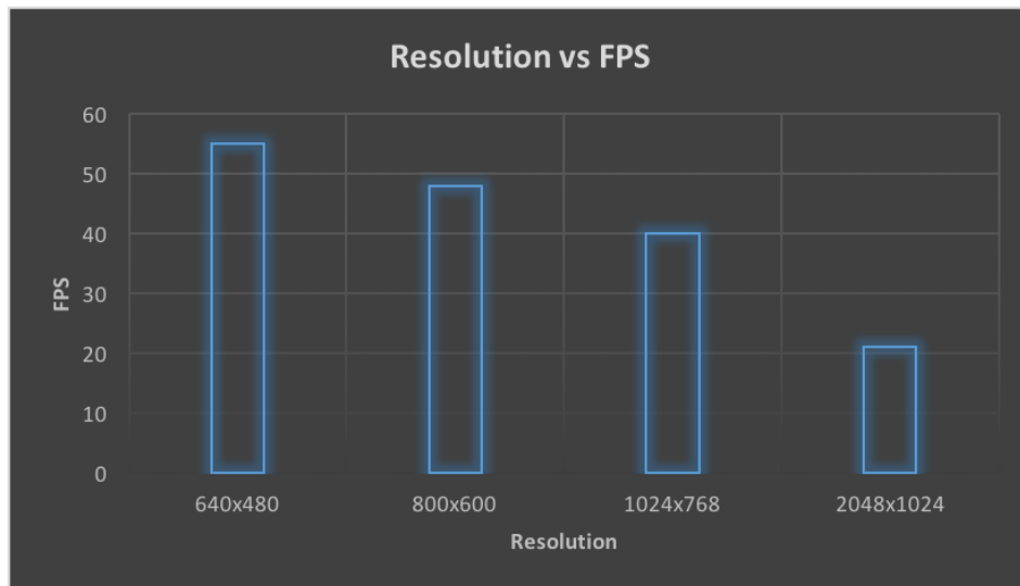
Figure 4.4: Each image is rendered with 5 samples and a step size of 10 on NVidia GeForce 940M with Altier model .
