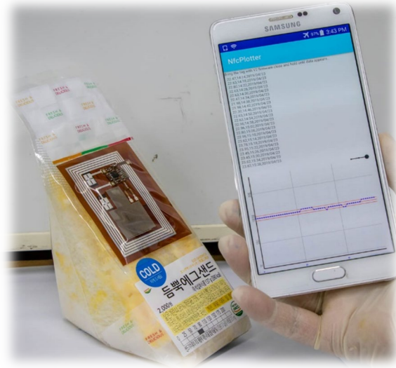
Figure 9 – Image of smartphone reading the temperature time history stored in the label
