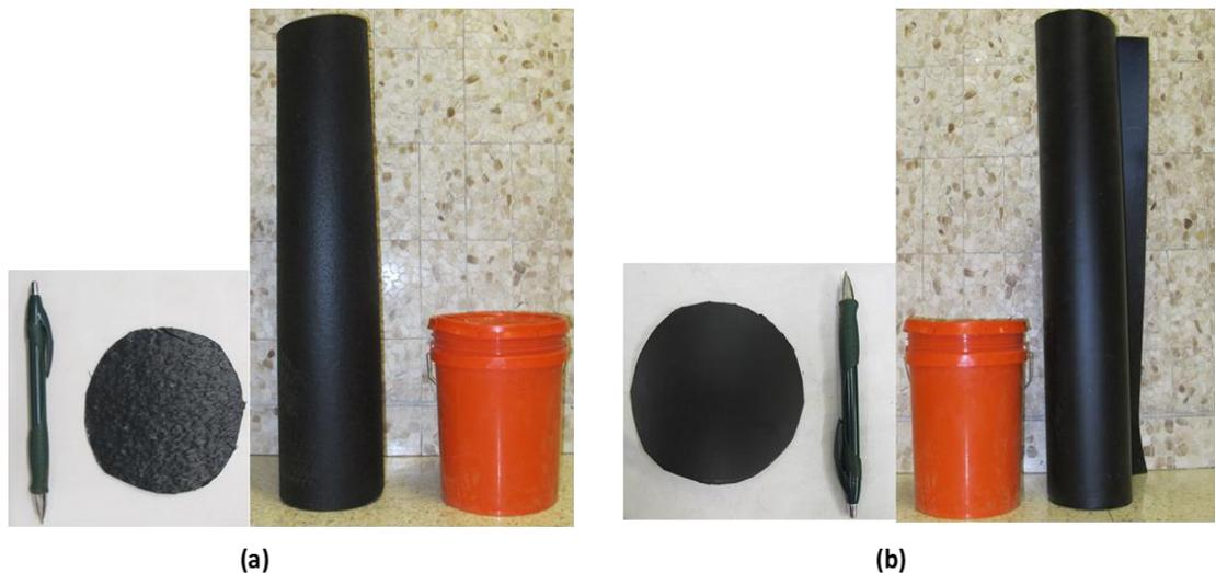
**Figure 3.1. Textured geomembrane cut and rolled (a) and smooth geomembrane cut and rolled (b)**
