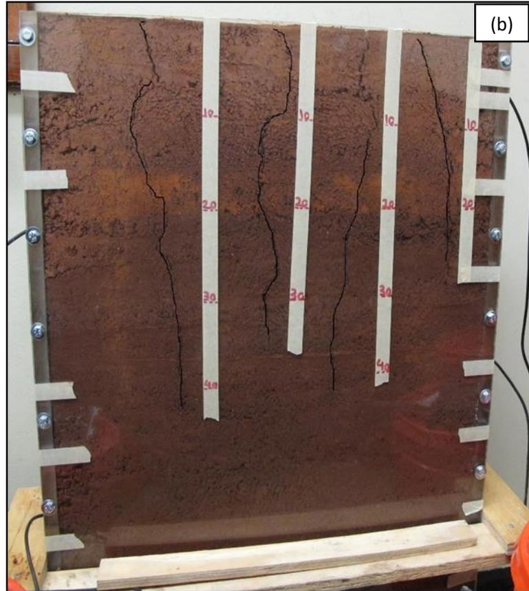
Figure 2.11. Desiccation crack depth measurement in the desiccation box, top view (a) side view (b)
