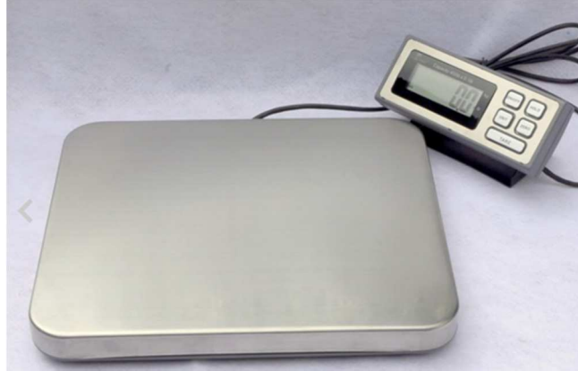
Figure 6. 17: A large digital scale is used for measuring the thrust values. [43]
