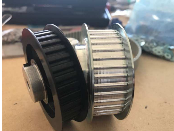
Figure 6. 8: A comparison between an AT5 and XL pulley. The AT5 pulley can be seen in the right part of the image, and XL pulley – in the left part of it.
