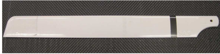
Figure 2. 13: This is a 325 mm length of helicopter rotor blade. It is made of carbon fiber composite material and commonly used on Trex-450 RC Helicopter. [20]
