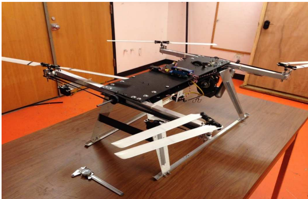
Figure 2. 9: A gas-powered variable-pitch quadcopter that was built by OSU senior design students in 2016. [18]
