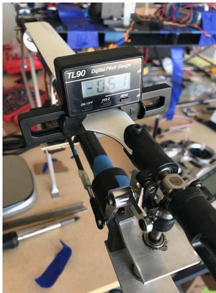
Figure 6. 11: Example of using a pitch gauge to calibrate the rotor blade pitch angle.
