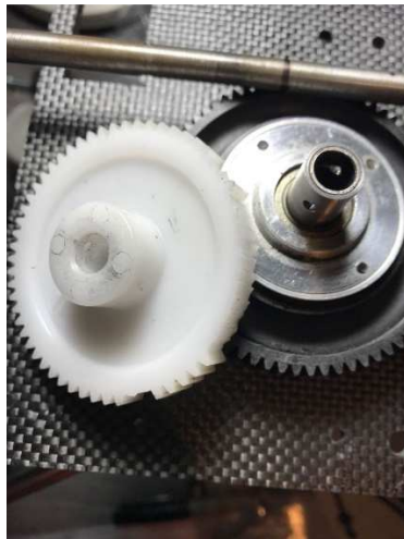
Figure 6. 5: motor gear damaged after the first testing
