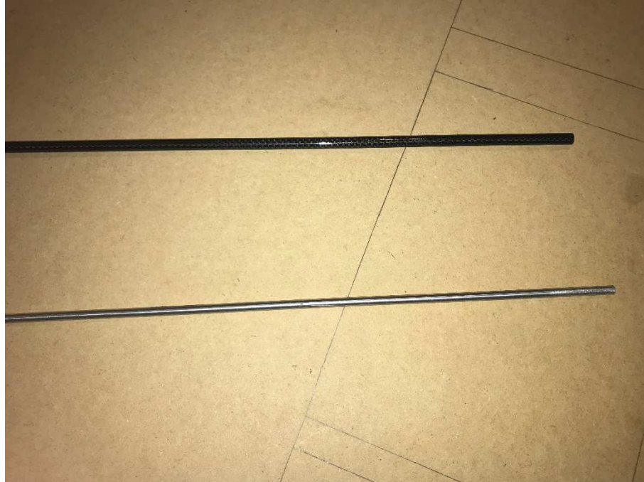
Figure 4. 27: The carbon fiber shaft is on the top, and the solid steel shaft is at the bottom.
