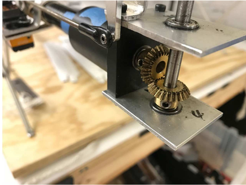
Figure 6. 23: A moderate bevel gear teeth wear on the rotor shaft bevel gears
