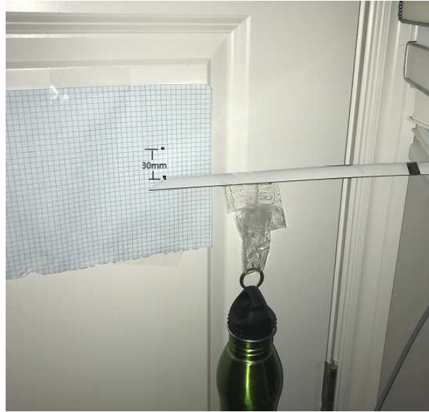
Figure 4. 13: Blade deflection test
