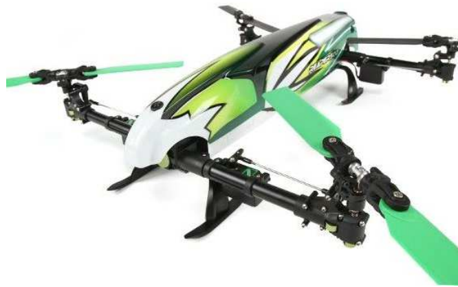
Figure 2. 6: RC variable pitch quadcopter made by Hobbyking. [19]
