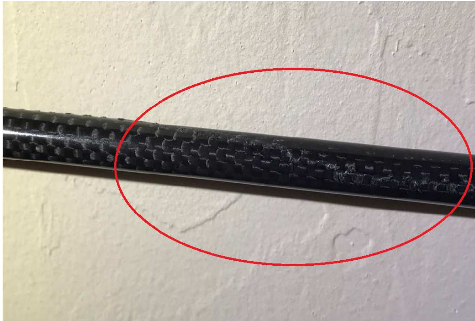
Figure 4. 31: Carbon fiber shaft failure under torsional load
