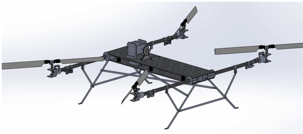
Figure 4. 1: The first design of the electricity-powered variable-pitch quadcopter. The power transmission system from the motor to the main shaft is a gear-driven system
