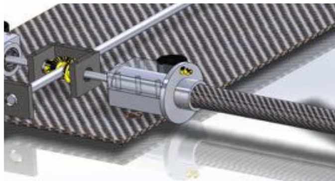
Figure 2. 18: A tilt rotor mechanism conceptual design by Logan
