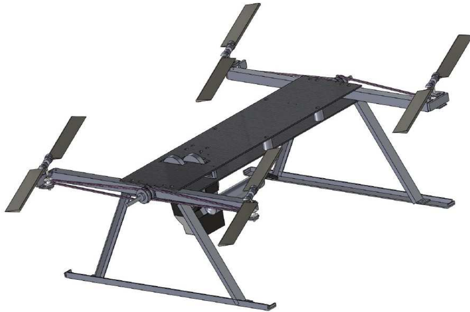
Figure 3. 2: Example of H-shape configuration variable pitch quadcopter [18]
