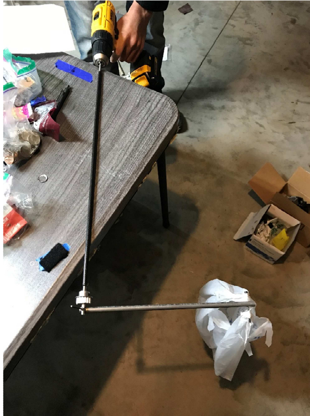
Figure 4. 30: A torsional test conducted on the carbon fiber shaft
