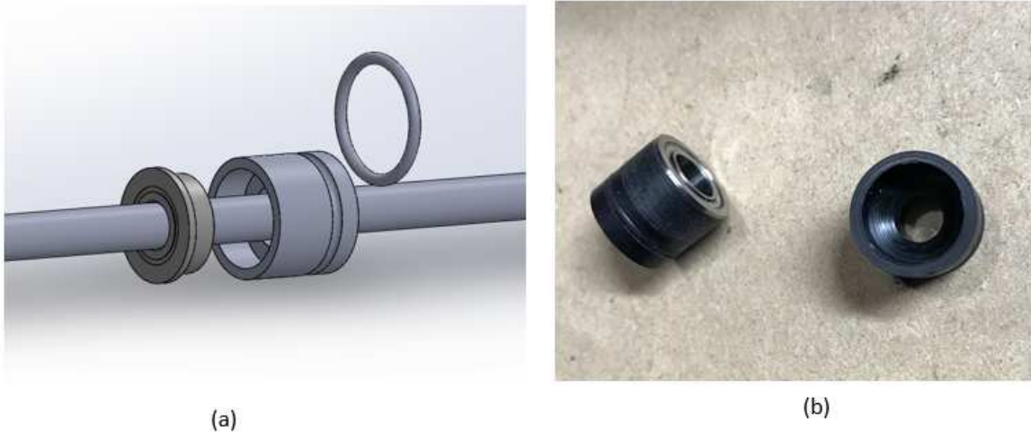
Figure 5. 14a and 5.14b: The figure on the left demonstrates assembly drawing of the bearing carrier. The figure on the right is the actual bearing carrier.
