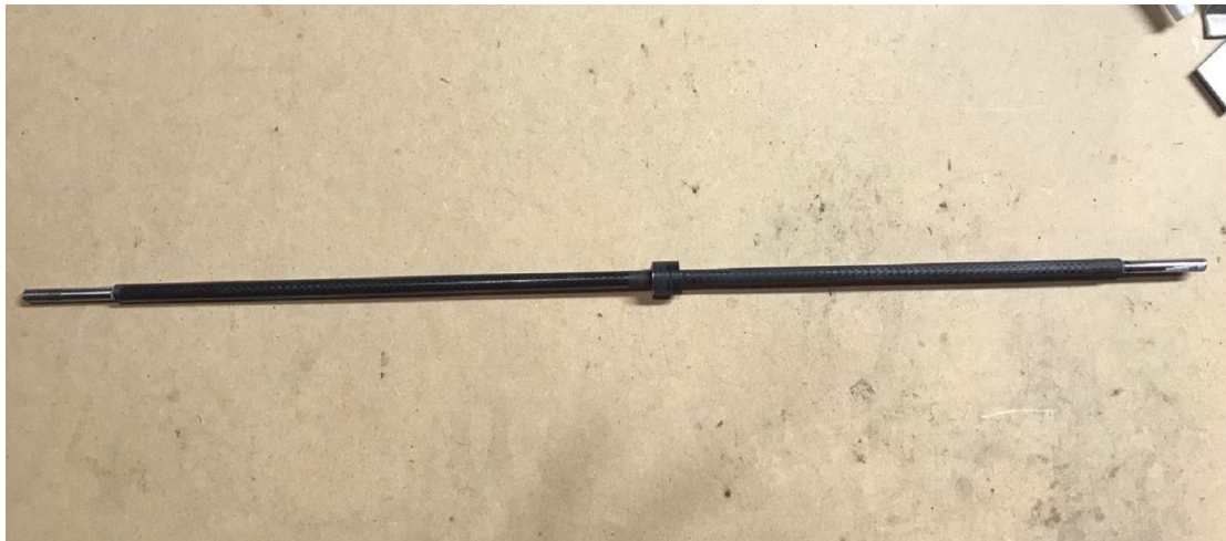
Figure 5. 15: Half of the carbon fiber shaft is sanded for fitting into the bearing carrier.
