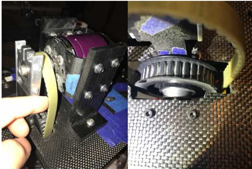
Figure 6. 7: The belt became loose, and the white powder accumulated on the pulley indicated the excessive belt wear caused by belt slipping.
