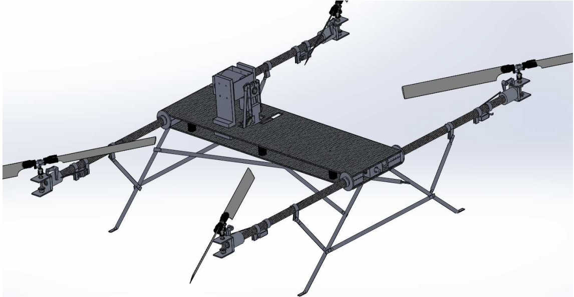
Figure 4. 2: The second design of the electric powered variable pitch quadcopter. The second design used the belt and pulley system to transfer the power from the motor to the main shaft.
