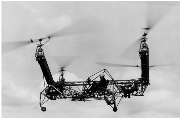
Figure 2. 3: Convertawings Model "A" Quadcopter [14]
