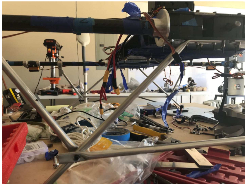
Figure 5. 8: Landing gear is constructed from the aluminum tubes
