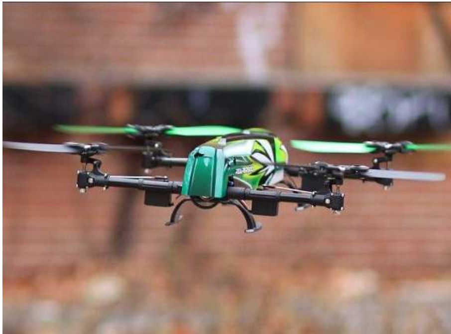
Figure 1. 1: Example of a RC variable pitch quadcopter from HobbyKing.[10]
