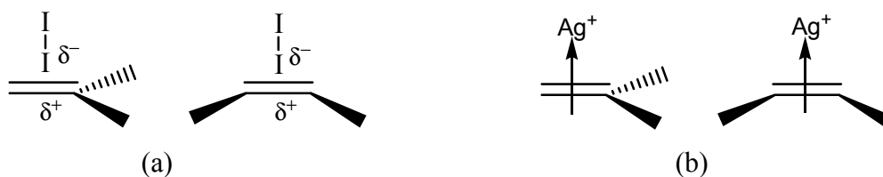
Figure 2-6. Sterically equivalent pairs of complexes in (a) complexation with molecular iodine and (b) silver ion complexation
